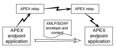
The APEX protocol is being developed in the IETF. It is very much based on the basic architecture of Internet email (SMTP, etc.) but has been designed as a general substrate for application data rather than just personto-person messaging.
